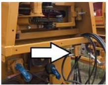
Hydraulic flow meter for manual control of tub speed and tractor load.
