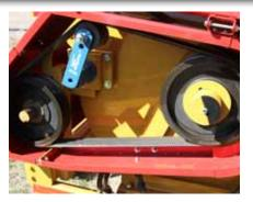
Durable belt drive systems to transition PTO power to the blower and hammermill.
