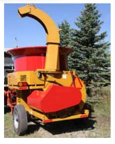
Feed discharges from grinder through a fan blower system with hydraulic adjustment vertically and 360 rotation for ease in feed placement.
